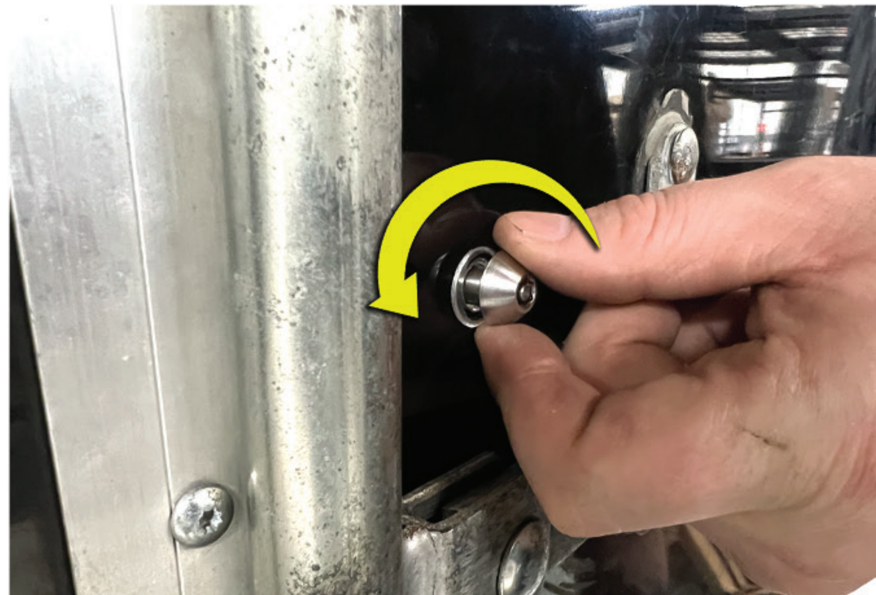
Turn the pin by hand and make sure it is threading into the anchor without cross threading. It may be necessary to realign the Lock Pin into the Anchor.
