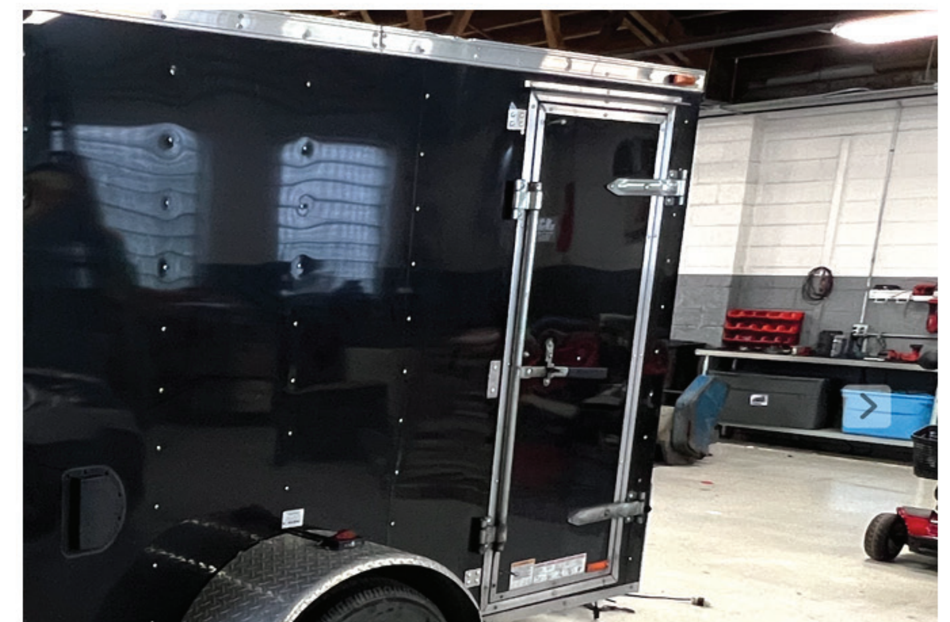
The Lock Pin is now in place securing the swing door. Note: The swivel bracket can be used on a variety of trailer doors.
