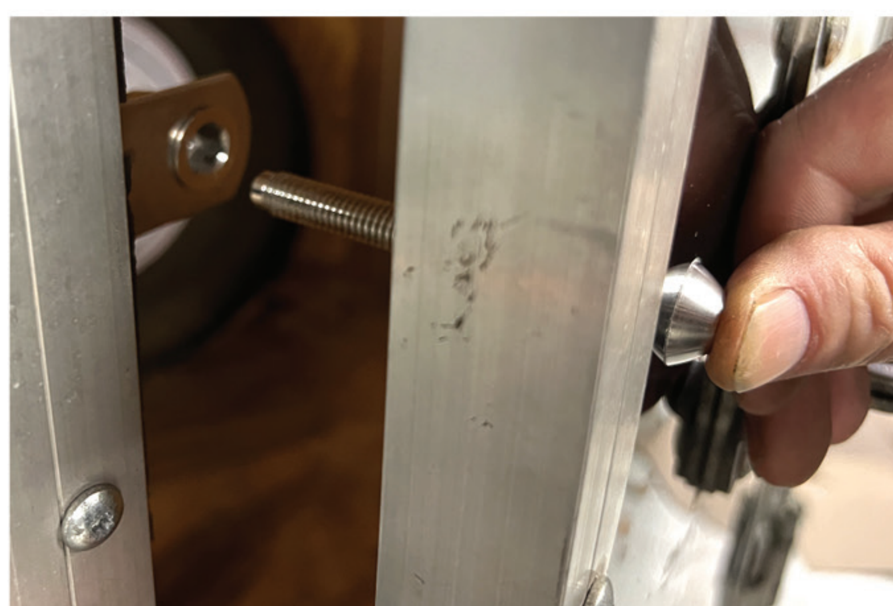
Insert the Lock Pin into the hole from the outside. Depending on the hole size the pin may need to be threaded in. If the hole is enlarged the pin will slide in/out easily.
