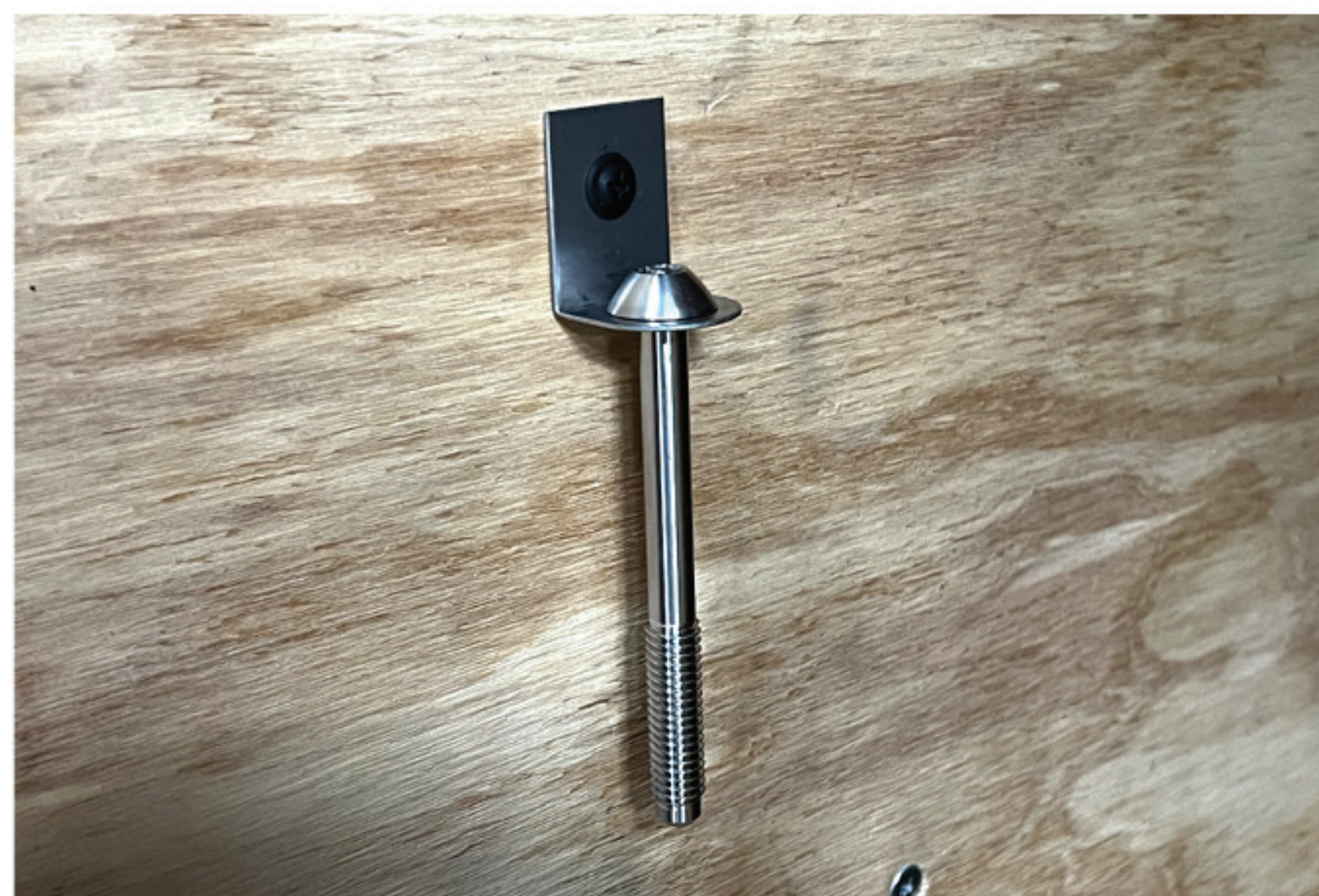
The Lock Pin can be stored in the pin holder when not in use.
