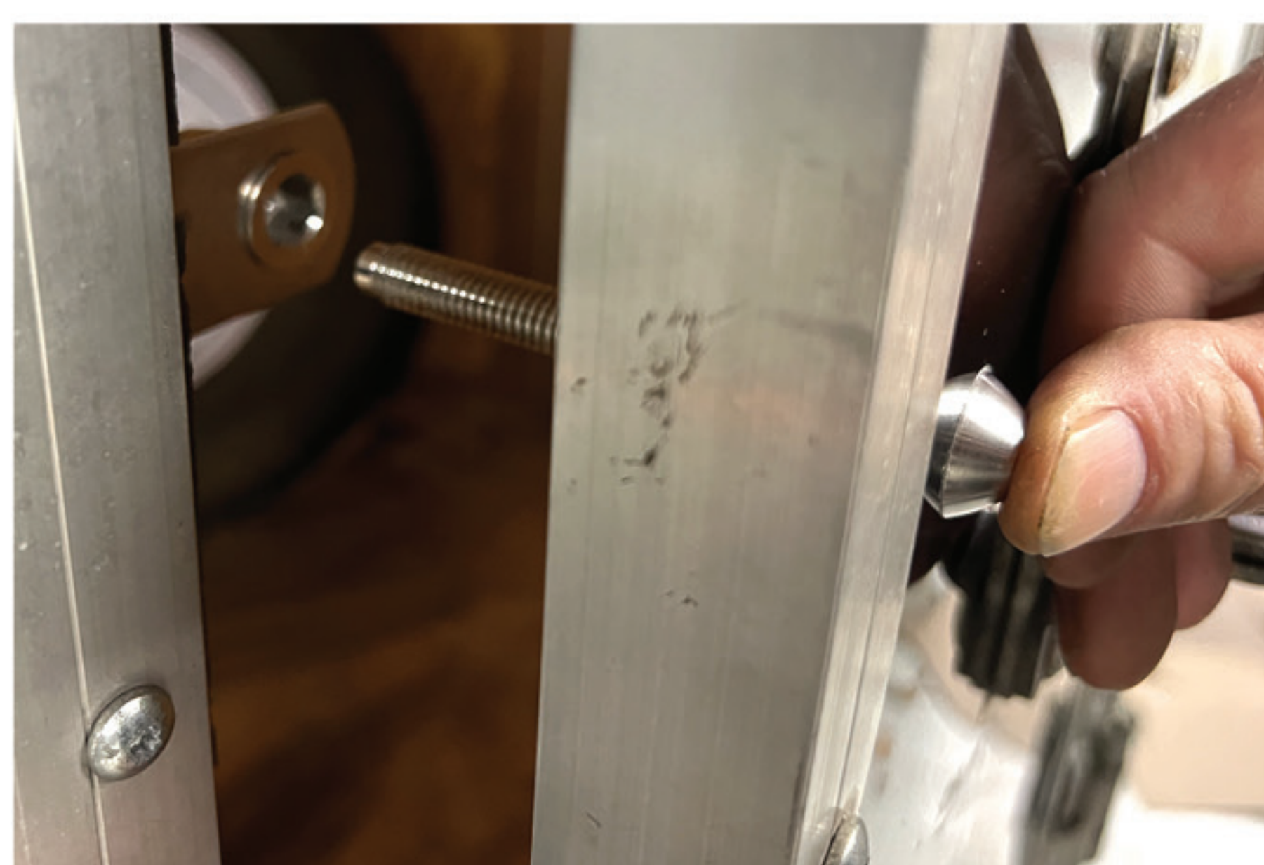
Insert the Lock Pin into the hole from the outside. Depending on the size of the hole it may need to be threaded in. If the hole is enlarged the pin will slide in/out easily.
