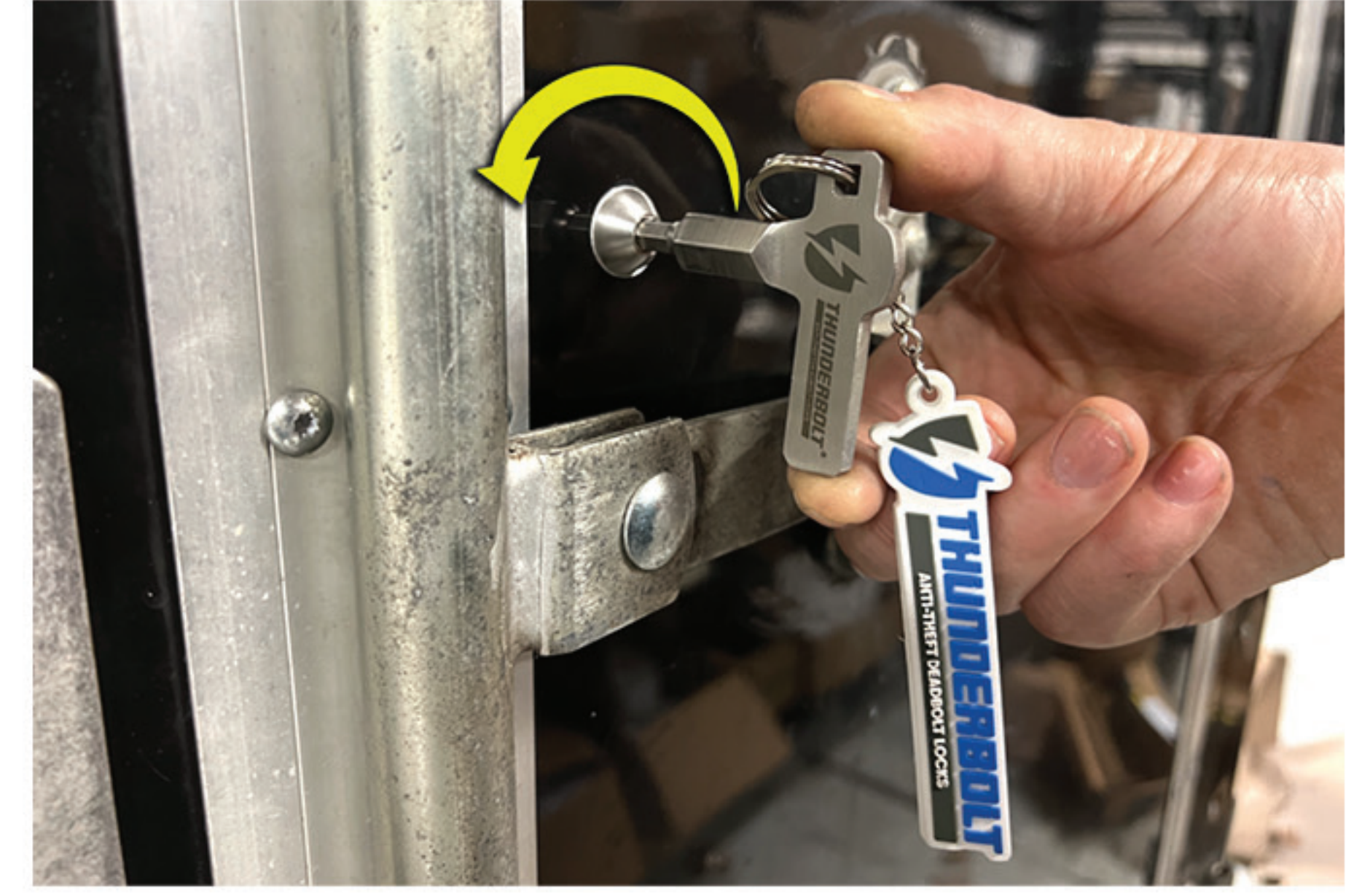
Tighten the Lock Pin using the Thunderbolt® Key Tool turning it to the LEFT. DO NOT OVER TIGHTEN.
