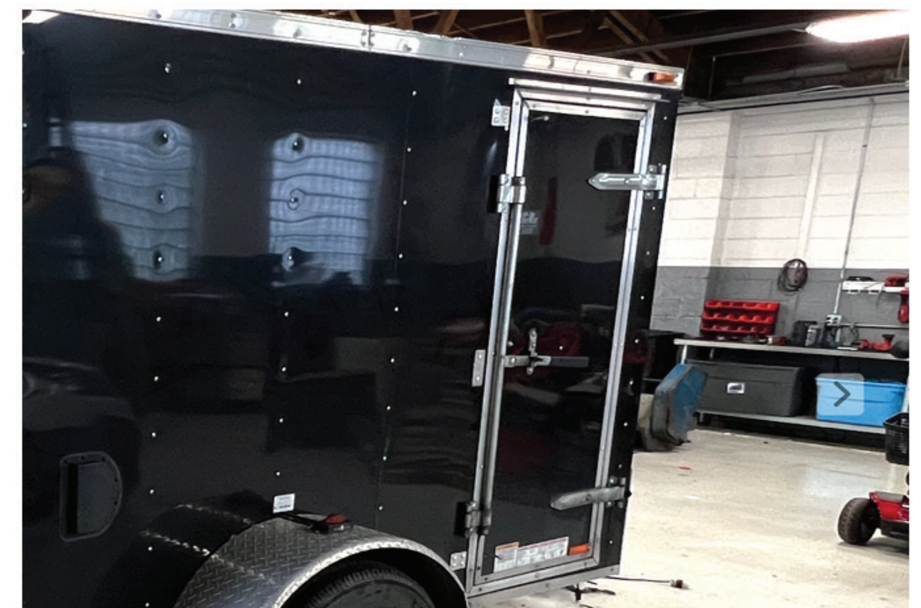
The Lock Pin is now in place to secure the swing door. Note: The swivel bracket can also be used on any swing or ramp doors.
