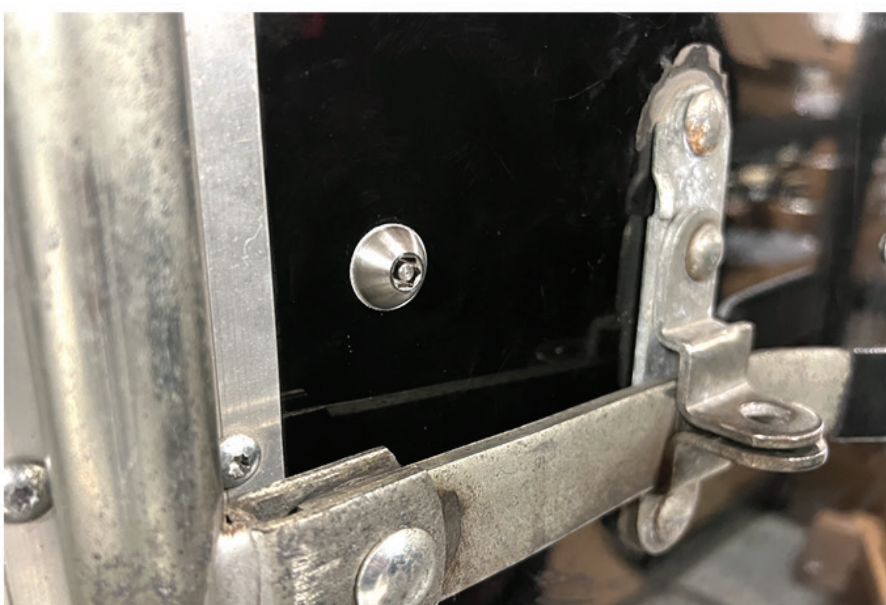
Additional Lock Pins can be installed on doors for added security. TIP: The bracket can be shimmed out to reduce the amount of threading when securing the pin.
