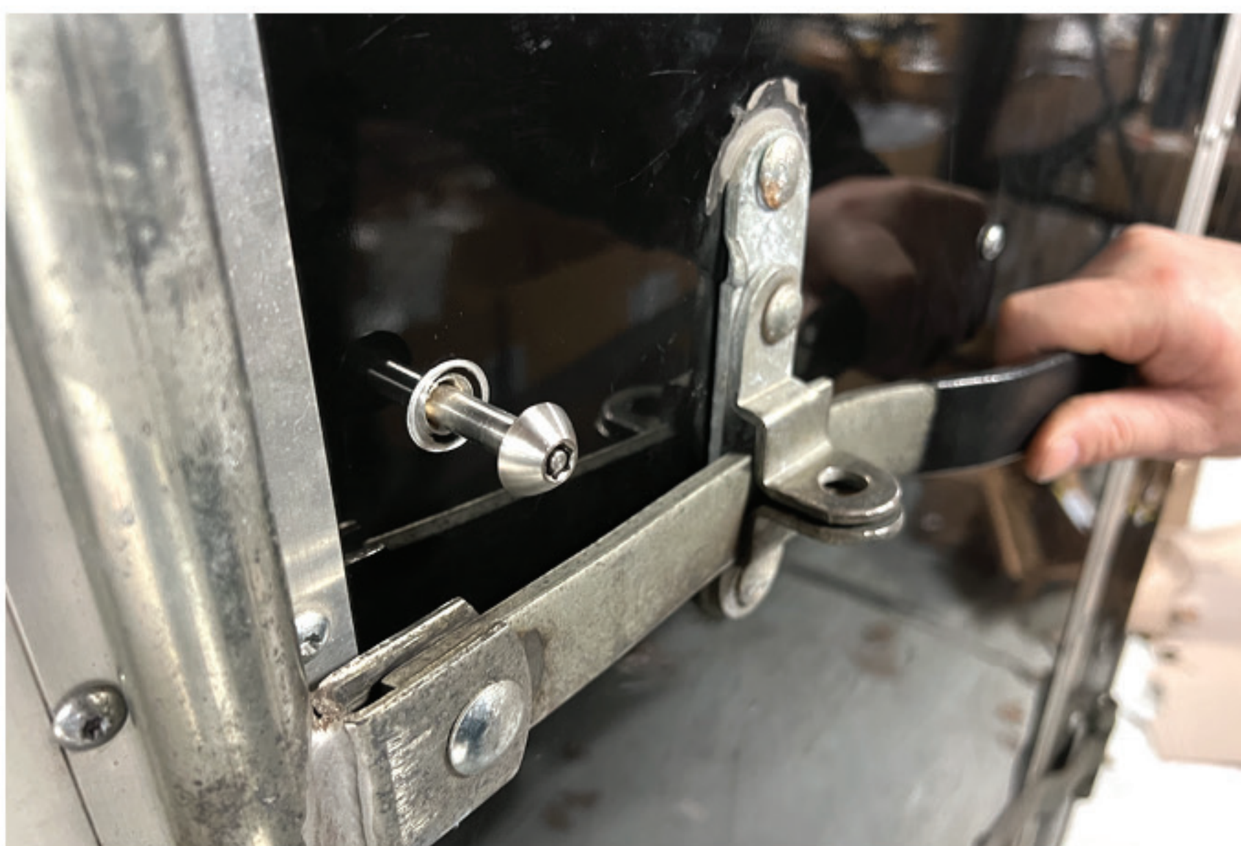
Shut and latch the door completely. TIP: A block or spacer can be used so that the swivel stays perpendicular each time it is moved into place.
