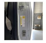
Front Cab Door "driver-side Raised Strike Bracket Location B-Pillar
