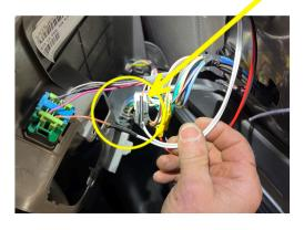
Always test your wires to be certain to locate the ignition wire. The ignition wire on this example van is green.
