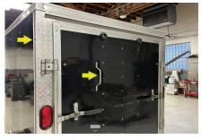
We suggest installing the Lock Pin on the side of the ramp door where the pull handle is attached.
