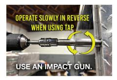
Place the LEFT-HAND Tap in the Socket from the Installation Kit. SLOWLY operate the Impact Gun in REVERSE to tap the hole.
