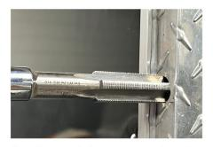
Once the threads have been cut, place the Impact Gun in the FORWARD position to remove the tap. Run the Tap SLOWLY back and forth to clean the thread a few times.
