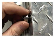
Hand tighten the Lock Pin by turning it to the LEFT. If there is any resistance enlarge or file the interior holes to fit.
