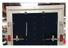
The Lock Pin is now in place to secure the ramp door. An additional Lock Pin can be installed on the other side for additional security.
