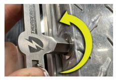
Turn the Anchor to the LEFT to thread the Anchor into the threaded hole. You can use pliers to help turn the key slowly, but use a rag to protect the key. Do not bend the key.
