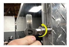
Insert the Thunderbolt® Key into the Anchor as the key doubles as a tool to thread the Anchor into position.
