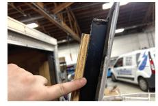
Locate a spot on the ramp door where the lock pin tip will engage into. The spot should align with the outside spot where the anchor will be installed.
