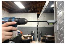
Drill a 3/16" hole from the outside spot all the way into the ramp door. Use the drill guide from the install kit to keep the hole as straight and accurate as possible.
