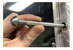
From the outside of the trailer insert the Lock Pin into the Anchor opening.
