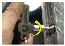
Tighten the Lock Pin using the Thunderbolt® Key Tool turning it to the LEFT. DO NOT OVER TIGHTEN.
