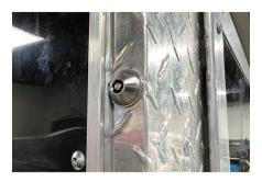
The Lock Pin is now in place securing the ramp door.
