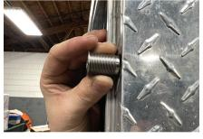
Fit the Anchor into the tapped hole using the collar guide at the tip of the Anchor. Keep the Anchor as straight as possible. Add a small amount of oil before inserting.
